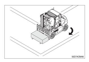
A Turn too sharp with a raised load and your truck can tip even at slow speeds. Travel with a load raised only when removing or depositing a load.
