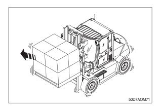
It should be observed that the side shift with load is operated in netural position before traveling.
